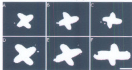
Fig 3. Binarized PLM images of the clover leaf pattern after 2.5 rev of 1.125" circular gels (A-C) and oval gels (D-F) at 0° (A, D), 22.5° (B, E), and 45° (C, F). Bar 1mm
